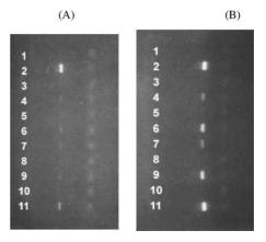
Fig. 5. Amplification efficiency: (A) HVS-IA amplifications (278 bp amplicon) and (B) L15997-H16071 amplifications (113 bp amplicon) with DNA extract from hair shaft of this Collaborative Exercise (11) and with other hair shafts extracts (4, 6, 7 and 9). Extraction blanks (3, 5, 8 and 10). Negative and positive controls (1 and 2).
